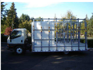
Complete 14 ½ Foot Contractor Glazing Truck, work ready fitted to Fuso cab chassis
