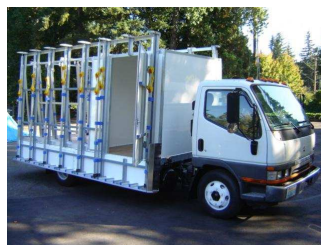
Complete 14 ½ Foot Contractor Glazing Truck, work ready fitted to Fuso cab chassis
