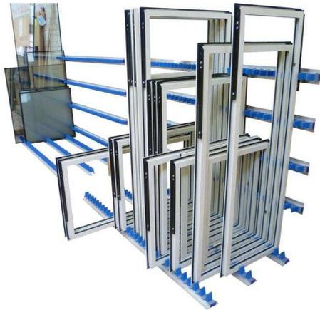
Many window companies are using our tooth system for storing IGUs, and increasingly the same technology is taking off for storage of sashes and door units.
