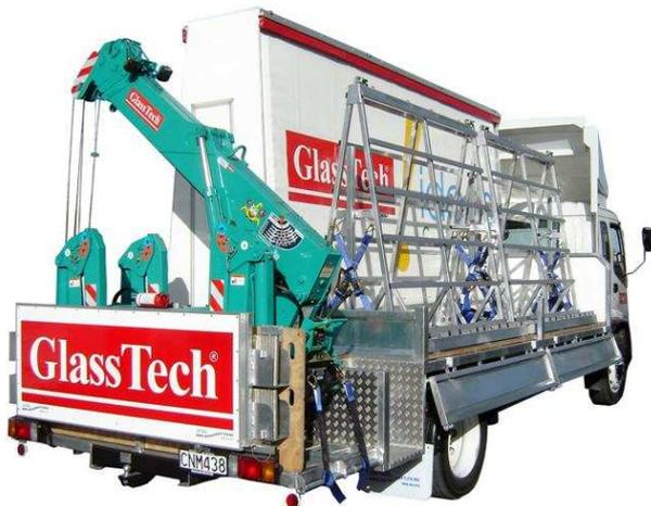
This crane truck, as mentioned in the Solar Glazing article, features a fixed A-frame rack for flat glass and solar panels, two lifting A-frames with certified lifting weights for lifting units into position on building sites, and a spider crane with ramps.
