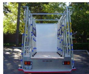
**Complete 14 ½ Foot Contractor Glazing Truck, work ready fitted to Fuso cab chassis**
