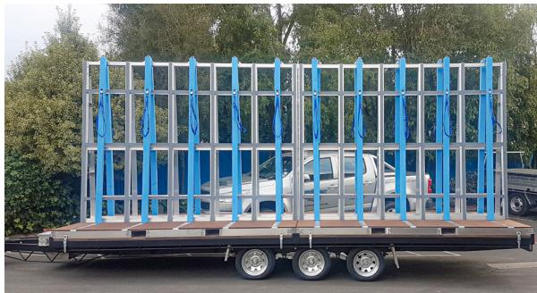
Demountable frames are lined with non-marking polymer foams at all contact points, ensuring that finished products are protected throughout transit.
