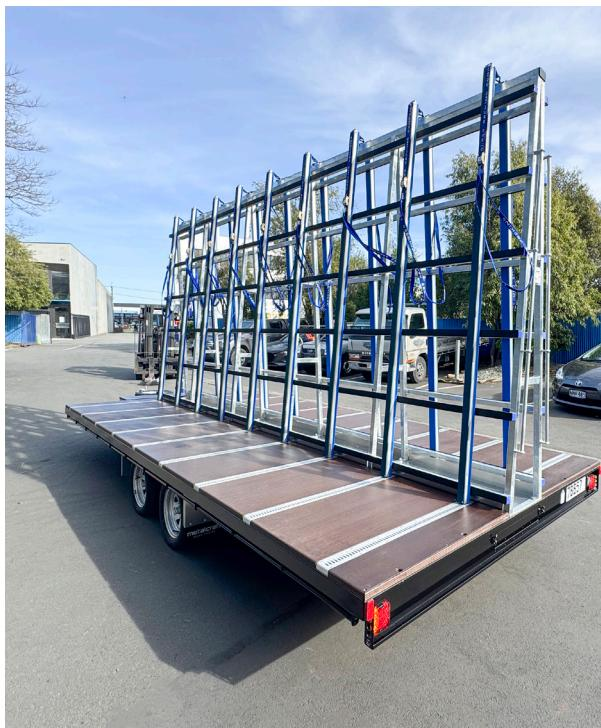
The trailer deck is clad in 28 mm hardwood container ply with inlaid slotted bases for secure positioning of poles from the Window Retention System. A 2.4 m pull-out ramp makes loading and unloading easier, while under-deck storage bins and integrated A-frame storage provide added practicality.
