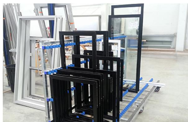
Teeth spaced with polymer to suite window sashes and doors.
