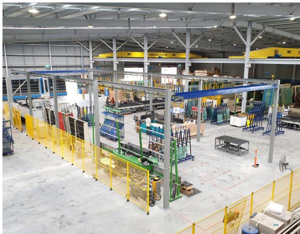
Our Light Rail Overhead Crane System is a freestanding structure designed for lifts up to 500kg, ideal for loading and unloading glass within a factory or dispatch area. The system combines German-designed Helm Technology tracks and running gear with a locally engineered and fabricated supporting structure, creating a cost-effective, tailored solution.
