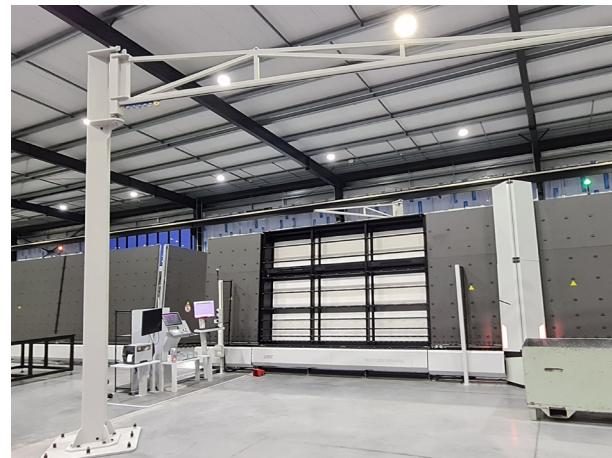
Jib cranes, also known as swing cranes, provide a cost-effective lifting solution for heavy glass items. They are commonly used beneath gantry cranes and are ideal for lifting items onto and off machinery or vehicles.
