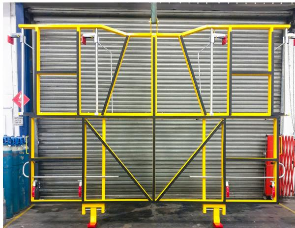
Packlifters are engineered to secure, lift, and transport entire packs of glass safely within a factory.
