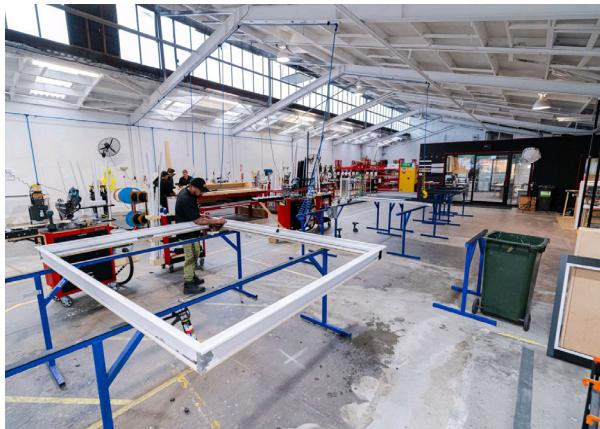
Our prepping tables have a solid 29 mm hardwood plywood tops – stay flat, resist wear, and provide a robust work surface. Polymer-clad bearing surfaces – protect flat panels from scratches and transit rub
