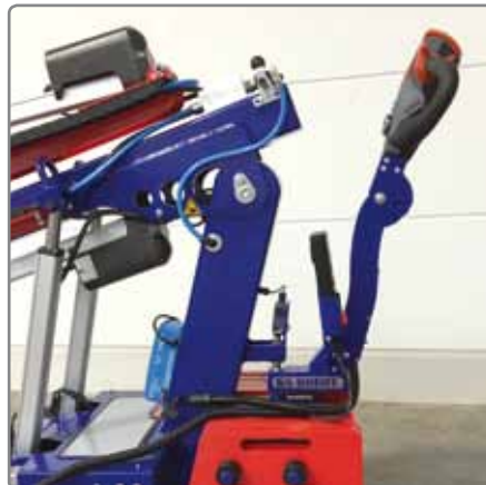
Foldable steering rod saves space
