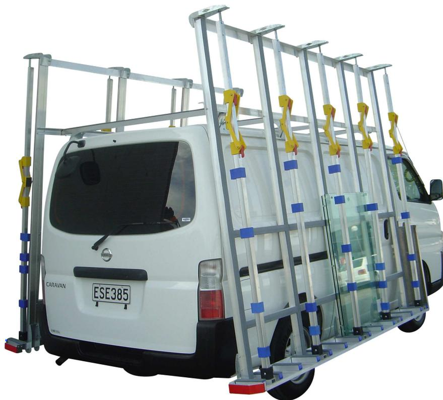
The Glass Racking Company van glass frail has been developed to assist glass companies, glaziers and window installers to transport flat glass to site. Options include internal and external racks, height extension, and scissor clamp load retention.
