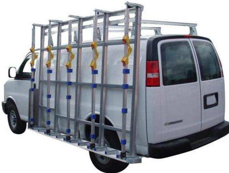
The Glass Racking Company van glass racks have been developed to assist glass companies, glaziers and window installers to transport flat glass to site. Options include internal and external racks, height extension, and scissor clamp load retention.
