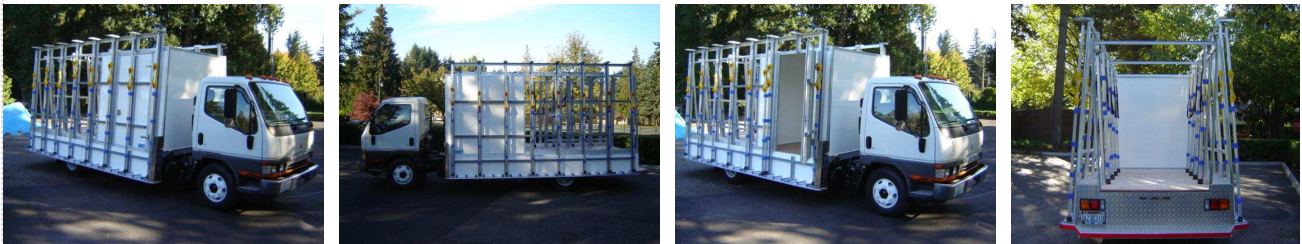
Complete 14 ½ Foot Contractor Glazing Truck, work ready fitted to Fuso cab chassis
