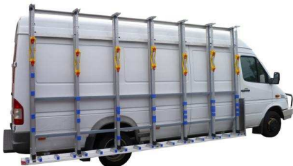
2.2M x 4.5M gutter clamped and height adjustable van rack
