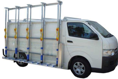
1.65M x 2.9M van rack with height extension up
