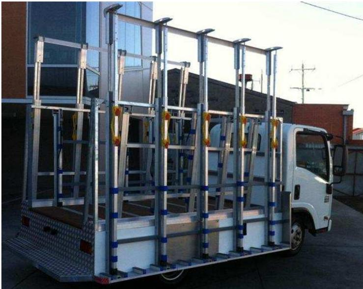
Southern Star Windows in Geelong are very pleased with their new glass truck. The cab chassis is an Isuzu Low Loader, and the dual side racks are both 3.2M long with 5 poles each. The external racks are both 2.2M tall with both sides being height extendable to 2.7M. All the external poles have scissor clamps.
